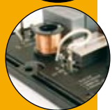
Configuration via cable jumpers
